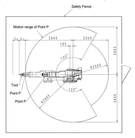
Figure above shows top view of robot, with robot mounted on shelf and facing sideways. The maximum motion range of the robot is based on point P. Safety fence dimensions must exceed the sum distance calculated as: maximum motion range of robot  $+ L_1 + L_2$ , where  $L_1$  is max. distance from B to tool tip, and  $L_2$  is distance for safety allowance
